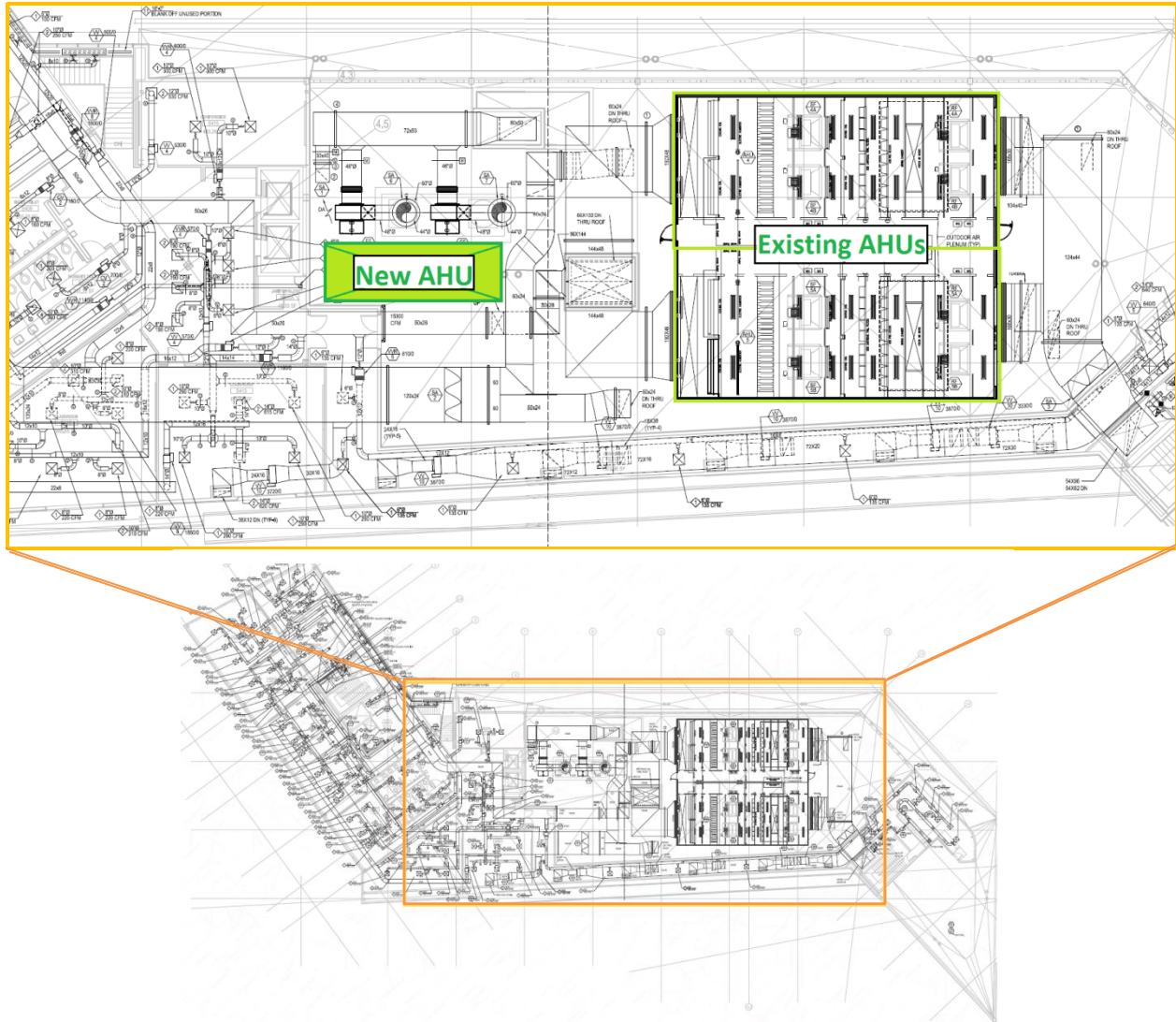
Figure 23: Roof Plan Showing Air Handling Unit Layout
